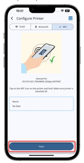
5. Hold the Android device or the iPhone near the printer's NFC antenna. The position of the NFC antenna is marked with a  $\P$  symbol.
