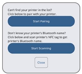
On the help dialog, tap [Start Pairing] to pair the desired printer. If you want to find out the Bluetooth name of your printer, tap [Start Scanning] and hold the iPhone near the printer's NFC antenna. The Bluetooth name of your printer is shown on the dialog.
