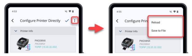
**For iPhones**, tap the *C* icon to reload the printer settings or the icon to save the printer settings to a file.
