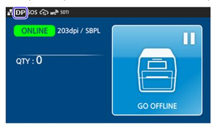
If the **DP** status icon is not shown, you can enable the direct print mode in the [SETTINGS] > [Applications] > [DIRECT PRINT] menu. Select the check box of [Enable] to enable the direct print mode.
